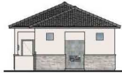
REAR ELEVATION ELEVATION B 1/8" = 1'-0"
